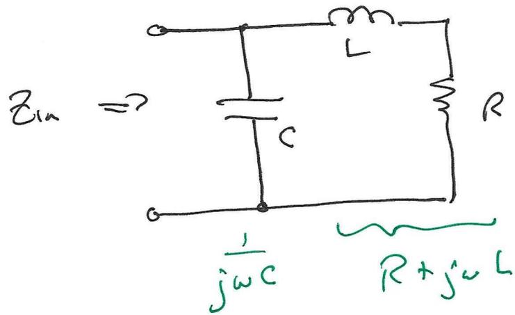
$$Z_{in} = \frac{\frac{1}{j\omega C} (R + j\omega L)}{\frac{1}{j\omega C} + R + j\omega L} = \frac{R + j\omega L}{1 + j\omega RC - \omega^2 LC}$$
