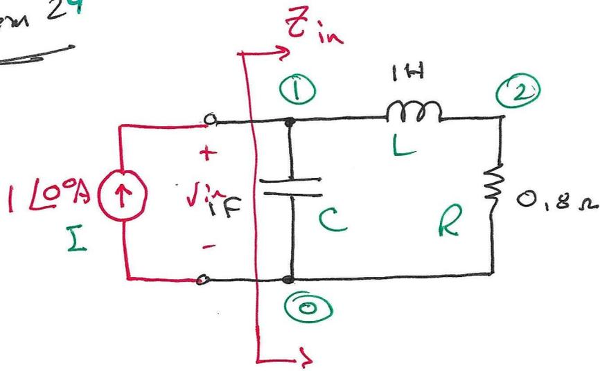
$$V_{in} = Z_{in} (1 \angle 0^\circ) = Z_{in}$$
