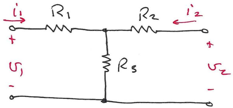
Find the impedance parameters  $Z_{11}, Z_{12}, Z_{21}, Z_{22}$
